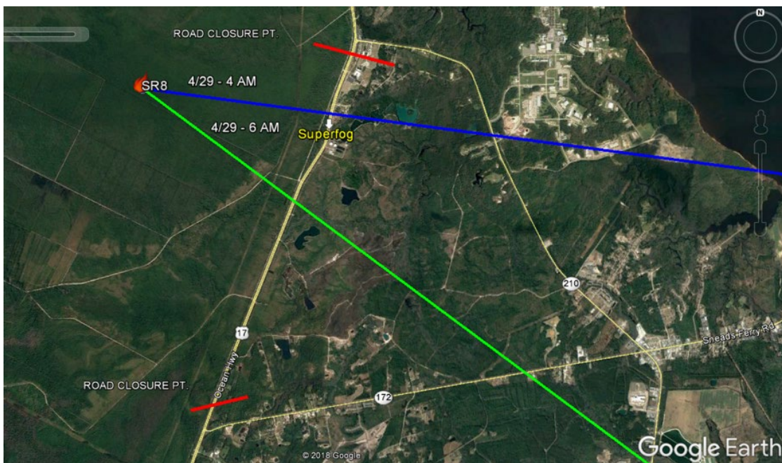
Figure 17. Modeled PC HYSPLIT 10 meter trajectories initiated for 4 AM (blue line) and 6:00 AM (green line) showing the probable center lines of the ground level smoke plume from an actual superfog event. At 6:15 AM Highway 17 North of Jacksonville NC was closed (red lines). Visibility was observed at less than 10 feet.
