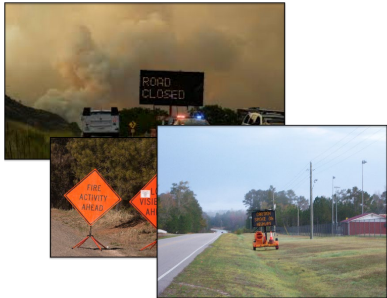
Figure 14. Examples of smoke signs and lighted boards.
