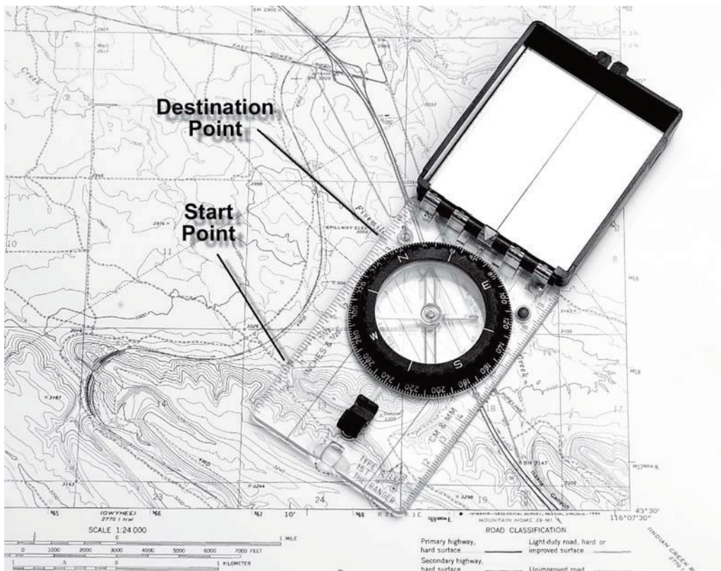
Figure 6-4. Measuring a bearing with a compass where the edge of the base plate touches both the start point (unimproved road) and destination point (lake that is east of spillway elevation 3008 point).
