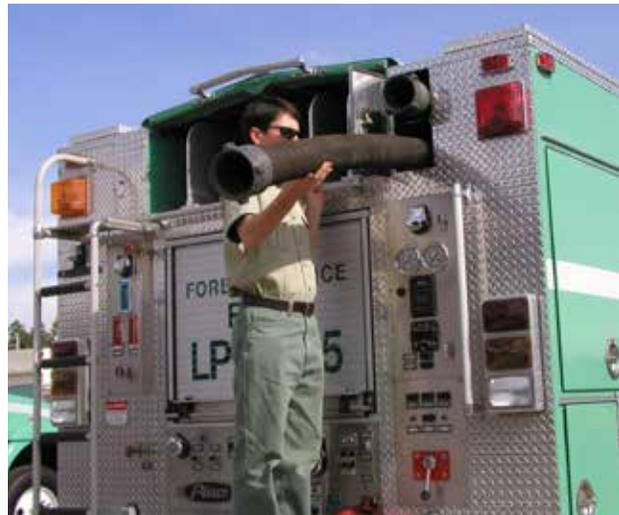
Hard suction draft hose is normally used on engines. The hard suction draft hose used is usually in 8- or 10-foot lengths, and ranging in diameter from 1 to 6 inches. Due to the inflexibility of the draft hose sections, storage methods vary. Draft hose normally is stored within a side compartment, or placed within external tubes or trays. A plastic or metal bin may be attached to the forward end of slip-on units for rolled suction hose storage.
