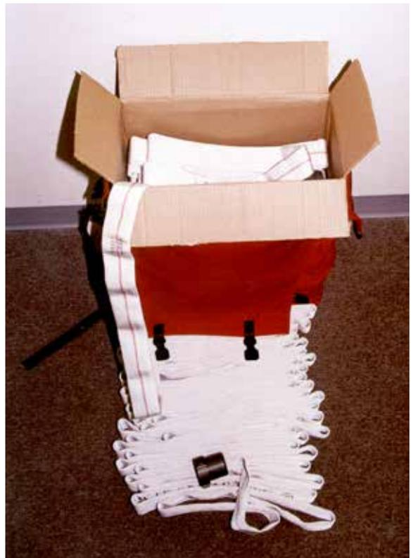
**Construction and material:** Cordura nylon outer pack with cardboard box inside to hold hose. The pack holds 400 feet of 1½-inch synthetic weeping hose. The hose is woven on a plywood jig and then inserted into a cardboard box. The cardboard box reduces the need to have every pack in the Cordura nylon outer pack. Once a box is used, it can be taken out of the pack and a full one put in. Approximate weight is 54 pounds.
