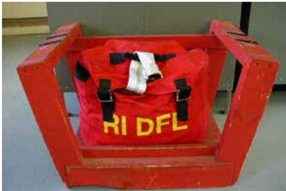
**Construction and material:** Hose rolled on a Rhode Island hose roller is opened and connected in a hose bag. Hose will then lay precoupled without kinking.
