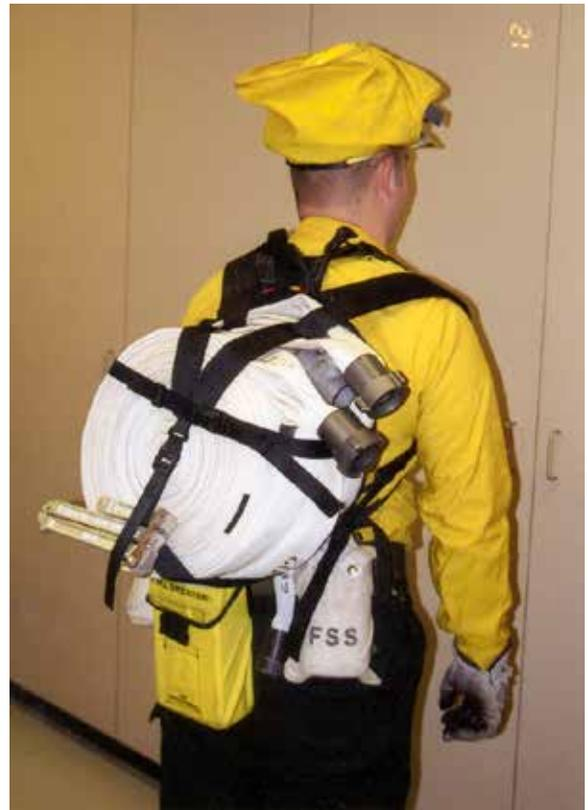
**Construction and materials:** Holds two 100-foot lengths of 1½-inch cotton jacketed hose or three 100-foot lengths of rolled synthetic hose. The pack is constructed of polypropylene webbing, 1,000 Denier Cordura, and acetyl buckles.
