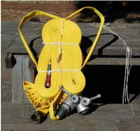
**Construction and materials:** Progressive hose lay that requires no packboard; stiffness of the hose is used as support. Hose is bound with tie-cords and shoulder straps are loops of hose. Capacity is 100 feet of 1-inch and 100 feet of 1½ inch fire hose.
