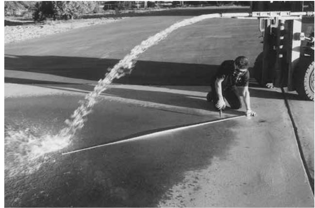
Figure C3—Splash test with 1½-inch pipe at suggested height of 54-1/4 inches; the calculated flow rate is 84 gpm.
