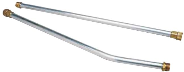
An applicator pipe, or wand, is available for reaching under logs, roots, stumps, and into the base of piled fuels. It can be used in deep duff, peat, and sawdust. The applicator is 52 inches long, comes apart in the middle, and has a 15-degree bend near the end. All connections are 3/4-inch GHT male threads to accommodate a special low-flow spray tip (3 gal/min with a 60 degree pattern). It is also a component of the Mop-up Kit.
