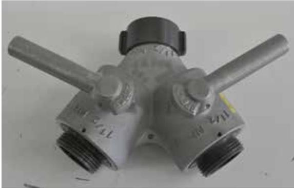
**Type:** Swivel inlet, gate valve branch outlets with handles.
