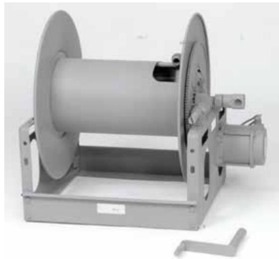
**Construction and material:** Constructed of steel or aluminum. Drum and rims may be open or closed. Swivel joint connection may be capable of operating at hydrostatic pressures of at least 600 psi. Rewind by hand crank, electric motor, or by hand using side rims. Brakes maintain position of reel and hose. Hose reel information is available from equipment suppliers. Normal use is with high-pressure rubber hose. Specify NH or NPSH hose threads and type of riser which can be hose-specific.
