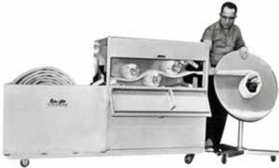
**Type:** Powered mechanical hose washer.
