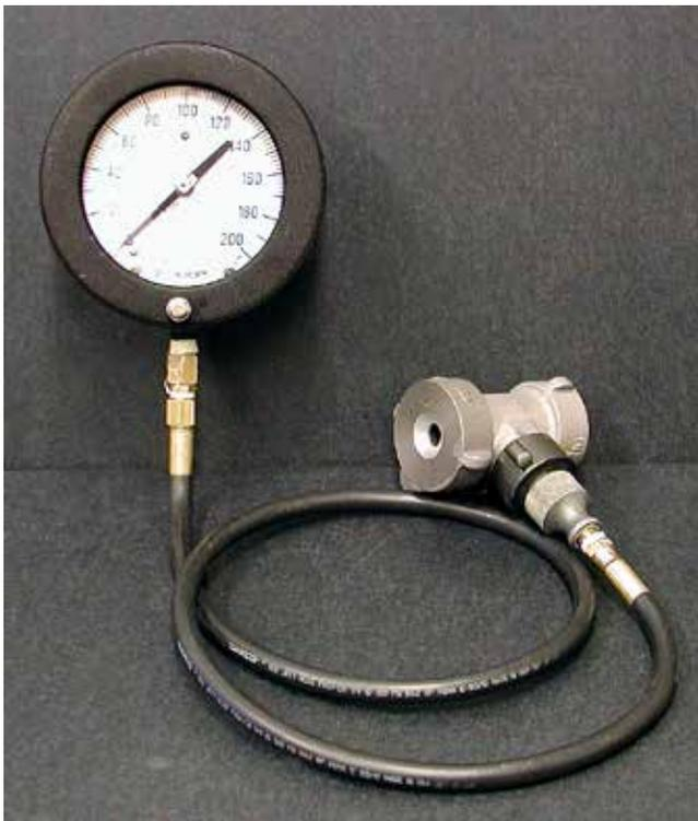
Figure C1—Photo of sharp-edged circular orifice system.
