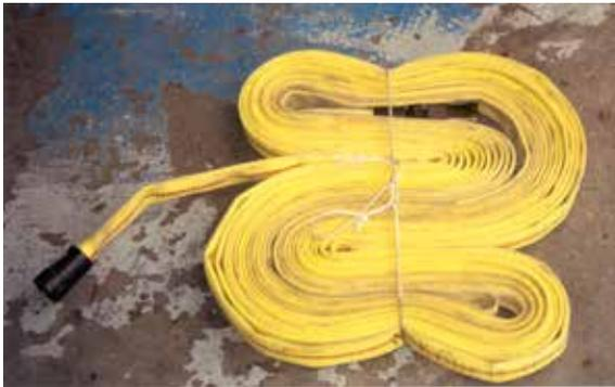
**Construction and materials:** Progressive hose lay that requires a heavy duty nylon duck packsack to harness 100 feet each of 1-inch and 1½-inch all-synthetic hose capacity. Total weight is 27 pounds.
