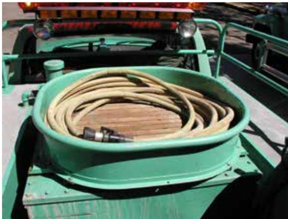
**Construction and material:** Constructed of steel sides, wooden duckboard on the bottom, and water repellent-type fabric cover with fire hose connected to the engine through a hole in the side of the basket. Capacity depends on size and type of hose. Normal use is 200 foot 1-inch single cotton-synthetic jacket lined hose. Hose basket minimizes rear view obstruction and has no moving parts.
