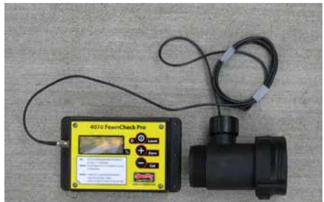
Figure 7—Portable foam concentrate meter.
