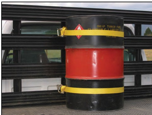
Figure 87: A drum that has been secured for transport.
