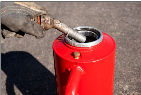
Figure 90: When a drip torch is filled properly, the pump nozzle touches the container, preventing sparks from static electricity generated by flowing fuel.
