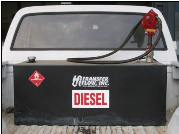
Figure 105: A small tank marked for transporting diesel.
