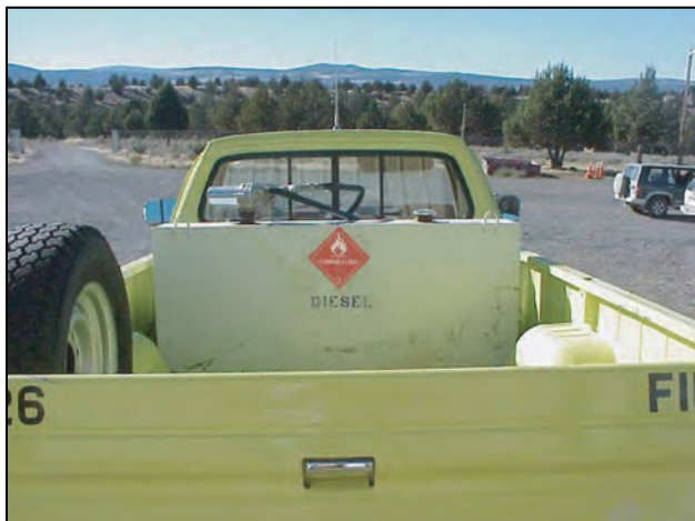
Figure 102: A typical non-specification tank used for transporting diesel. This photo has been digitally manipulated to show the proper DIESEL marking.
