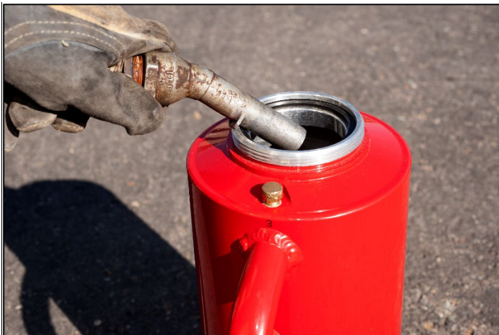
Figure 101: When a drip torch is filled properly, the pump nozzle touches the container, preventing sparks from static electricity generated by flowing fuel.
