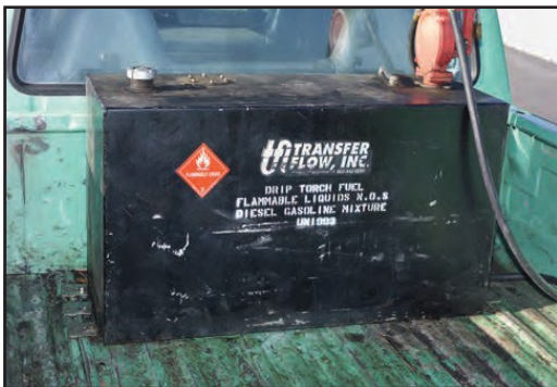
Figure 97: A Transfer Flow tank marked for drip torch fuel.
