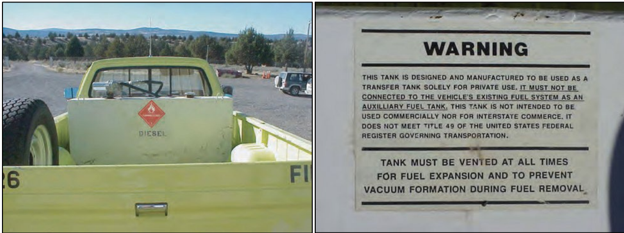
Figure 25: A typical non-specification tank (left) for transporting diesel. Note the label (right) warning that this tank does not comply with regulations for transporting gasoline. Regulations do not require a DOT-specification tank for transporting diesel. This photo has been digitally manipulated to show the DIESEL marking.
