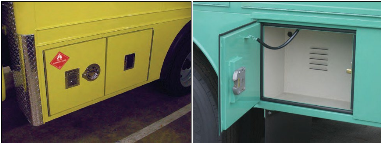
Figure 109: Examples of vented compartments for carrying fuel. The photo on the left shows the vent on the outside of the vehicle. The photo on the right shows the vent on the inside of a compartment used to carry fuel containers.
