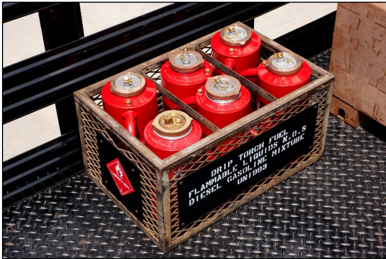
Figure 44: Drip torches secured in a rack.
