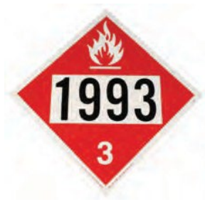
Figure 32: A FLAMMABLE placard with the identification number included.
