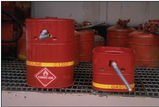
Figure 50: Safety transport cans showing the colors required by OSHA and the proper markings.
