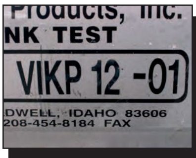
Figure 98: Tank inspection markings on a DOT-406 tank. This tank was last inspected during December 2001.
