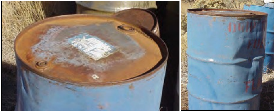
Figure 86: A drum that should not be reused because the head is bulging (left) and the side is dented (right).
