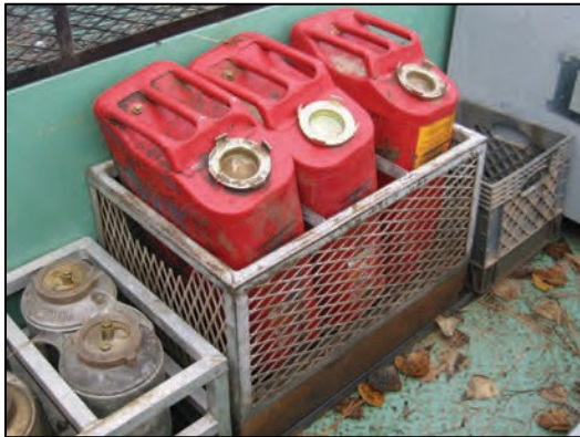
Figure 59: Fuel tanks for the Mark 3 pump secured properly for transport.
