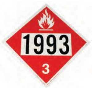
Figure 43: A placard with the UN identification number for drip torch fuel included. When the identification number is not included in the placard, a separate identification number (see Figure 31: A FLAMMABLE placard with a separate identification number.) must be with the placard.
