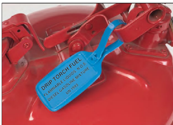
Figure 64: A safety can marked properly for transporting drip torch fuel. Because safety cans do not meet the UN specifications for safety transport cans, fewer can be transported at a time.
