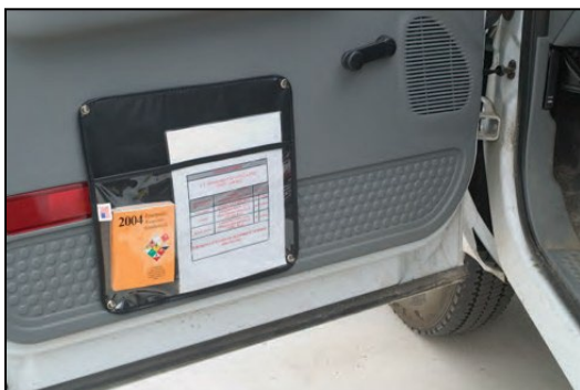
Figure 34: An example of an appropriate storage location for shipping papers and the ERG .
