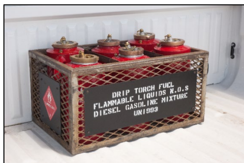
Figure 41: This rack is marked properly for transporting drip torches.
