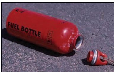
Figure 77: An aluminum fuel bottle that failed because it was overfilled.
