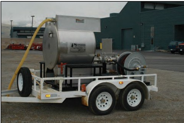
Figure 24: A 240-gallon DOT-406 tank being used as a batch mixer.
