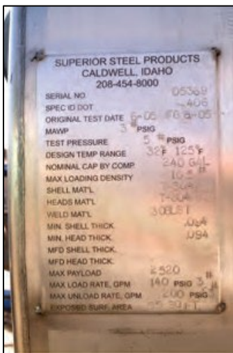
Figure 94: A label plate from a DOT 406 tank.
