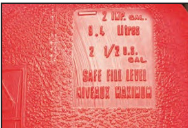
Figure 73: The fill line molded into a consumer plastic fuel container.
