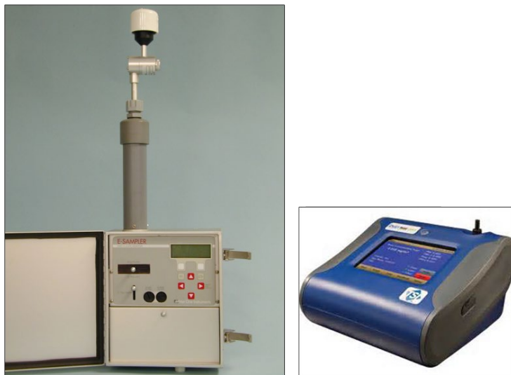
Figure 5.4.3. Nephelometers, such as the MetOne E-Sampler and TSI DustTrak, measure how much light is scattered by suspended particles in the air.
