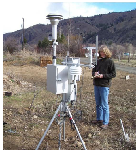
Figure 5.4.4. Beta attenuation monitors, like the rugged and portable E-BAM, are accurate and well-suited for smoke monitoring applications.
