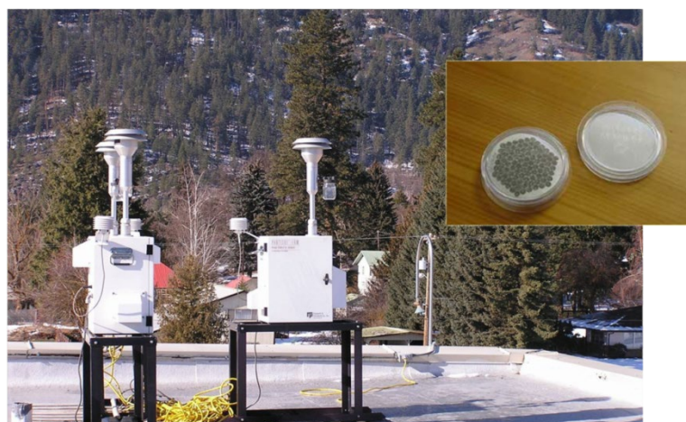
Figure 5.4.2. Gravimetric, or filter-based, monitors collect particulates on a filter that is weighed before and after the sampling period. This is the most accurate but also the most difficult way to monitor air quality.
