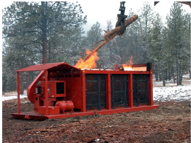
Figure 4.2.8. Air curtain incinerators result in very hot and efficient fires that produce little smoke.
