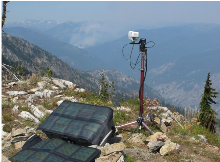
Figure 5.4.6. A solar-powered automatic camera that transfers images to a public or private web page can be useful for visually tracking plumes and smoke accumulations.
