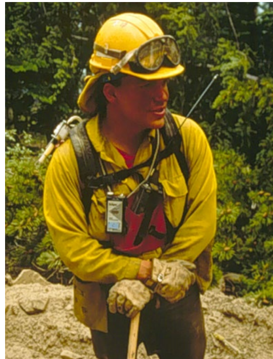
Figure 2.2.2. Backpack sampler capturing particulate matter, acrolein, formaldehyde, and other smoke exposure compounds within several inches of a workers face. Note the electronic dosimeter for testing.
