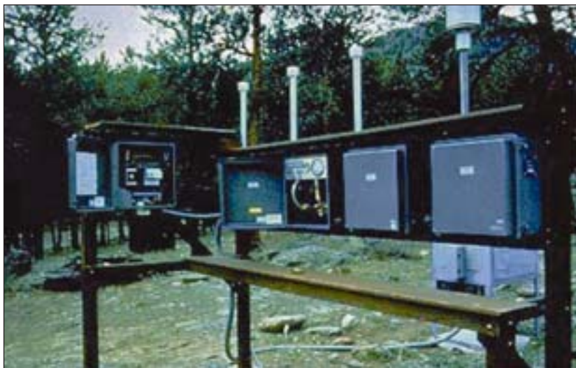
Figure 10.3. A typical IMPROVE monitor installation.
