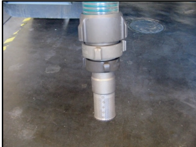
Figure 2. Foot valve attached to suction line with various adapters as needed to adjust for foot valve size.
