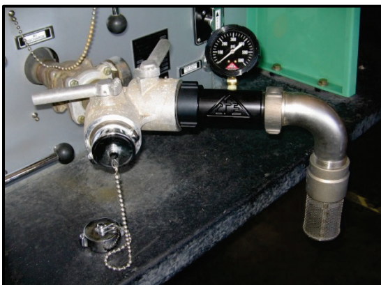
Figure 3. Pressure valve attached to the foot valve.
